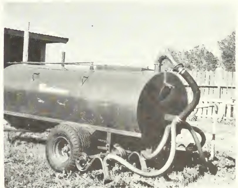
Figure 3.5.37 Vacuum tank-type wagon equipped with soil injector (courtesy Engineering Division, B.C. Ministry of Agriculture)
